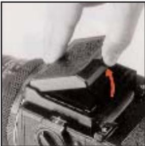
A. The focusing hood of the waist-level finder is opened by pushing or pulling up on the focusing hood/magnifier catch at the rear of the folded waist-level finder.
