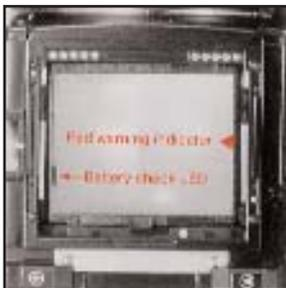
B. When set for multiple exposure, a red warning indicator will appear on the right-central area of the focusing screen.
