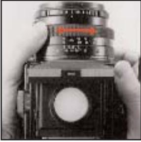
The lens is focused on the subject, by rotating the focusing ring in either direction, while checking the effect on the matte surface in the center of the focusing screen.
