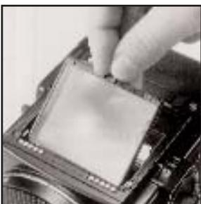
B. To install the focusing screen, insert the protrusions at the forward end of the focusing screen frame into corresponding openings in the focusing screen frame of the main body. Then, drop the rear end of focusing screen and slide the screen removal lever to the right.
