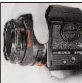
B. To detach the lens, rotate the lens in the clockwise direction while depressing the lens release button until the lens makes a full stop, at which point it can be detached.
