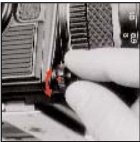
B. Safety Lock- The safety index on the shutter release button can be rotated to three positions for obtaining different shutter function. The settings are directly left, 45 degrees up from the side position and directly above, which have different safety lock functions.
