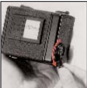
I. The film back winding crank is used for advancing the film, when the film back is detached from the main body for film loading. The film back winding crank can continue to rotate, even when the film is set for the first exposure. It should be rotated 2 or 3 times more, in order to take up any slack in the loaded film.
