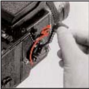
Rotating the film winding crank once, in the forward direction, will advance the film one frame and, at the same time, cock the shutter, with the winding action stopping automatically. Or, short, rapid strokes, up to an accumulated full rotation, will also do the job.
