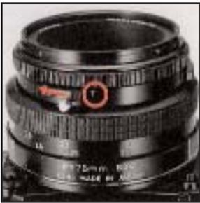
B. Next, cock the shutter with the film winding crank and then shift the time exposure lever to the left (looking from the body towards the lens) which will expose a red-colored "T" on the barrel. The shutter will stay open when the shutter release button is depressed in this condition. The shutter is closed by shifting the time exposure lever in the opposite direction and exposing the letter "A" once more.
