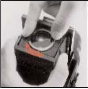
D. The standard magnifier supplied with the waist-level finder has a power of -1.5 diopters, which can be exchanged for others with powers of -4.5, -3.5, -2.5, -0.5, +0.5 and +1.5 diopters. These optional accessories should be purchased to suit the user's eyesight, if necessary. Simply rotate the magnifier frame in the counter-clockwise direction to unscrew. Attach in the reverse manner.
