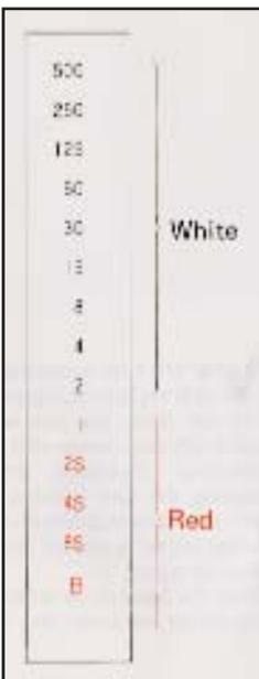
B. The numbers on the shutter speed scale are divided into red and white colors. Red-colored numbers are full number settings of 1 second and longer while white-colored numbers are from 1/2 to 1/500 second.
