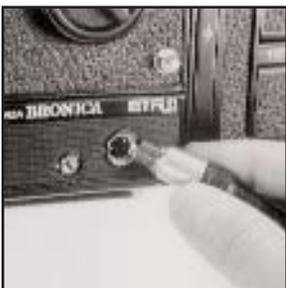
C. When a special SCA adapter is used in combination with the Zenza Bronica ETRSi, automatic flash adjustments are based on direct exposure readings made at the film plane. When the electronic flash unit is fully charged, a flash ready indicator will light up on the focusing screen.
