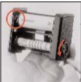
E. Rotate the film back winding crank on the right side of the film holder in the direction indicated by the arrow, while checking the advancing film. When the starting point, or arrow mark is aligned with the triangular start-mark on the top left side of the film holder, stop rotation.
