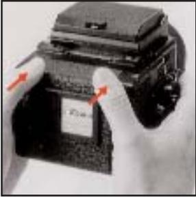
G. Close the back cover, by pressing firmly against the base of the film back, as illustrated. The back cover will automatically close and lock, with the safety lock also locking the back cover release button. The same operation will close the back cover when the film back is detached from the body.
