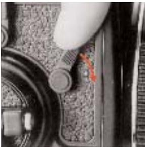
\* Rotating the film winding crank, after the 15th (120) or 30th (220) exposure when the mirror is locked up, will not advance the film as in the normal case, but will result in releasing the shutter once per 360° wind. Therefore, always return the mirror lock-up lever to the normal position after completing 15 or 30 exposures, before advancing the film to the take up spool.
