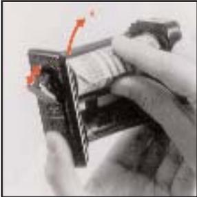
C. There are two spool holders on the film holder, with the top for the fresh film spool and the bottom for the take-up spool.
