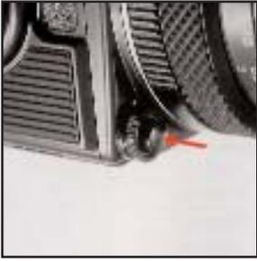
A. Depress the shutter release button with the ball of the finger. Press all the way in with a smooth and gentle action.
