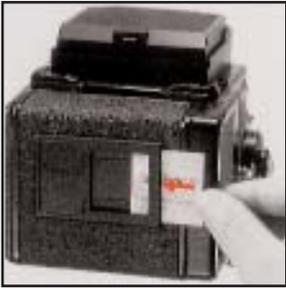
Upon loading the film, tear off the end flap from the empty film package and insert it in the film type indicator frame. This will help you keep track of the film loaded in the film back and should prove useful when two or more film backs are used, with different types of films.
