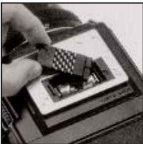
B. Coincide the plus (+) and minus (-) marks on the battery with similar polarity indications in the battery chamber. Then, push in the negative end of the battery first and follow with the positive end.
